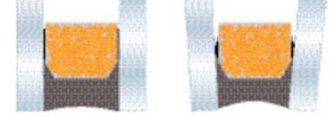
the glass/spacer bond places the primary seal in jeopardy of failure.
