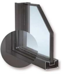
The flexibility of the Thermo Plastic Spacer allows for expansion and contraction without concentrated stress on the primary seal. The entire TPS spacer/seal expands.
