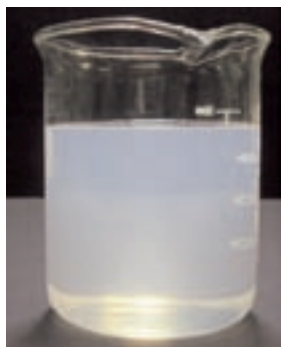
Picture 2: 1% Magnasoft JSS hydrophilic Textile Enhancer water solution after boiling at 100°C, pH: 12.
