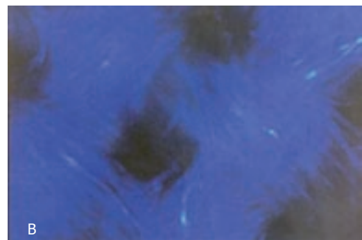
Picture 4: Micrographs of 100% cotton woven: A) untreated, B) fluorescently labeled Magnasoft DerMa NT textile enhancer visualizing the homogeneous treatment of fabrics.
