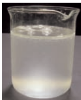
Picture 1: 1% Conventional amino silicone softener emulsion after boiling at 100°C, pH: 12.
